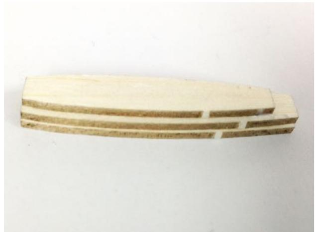
Oil Cooler - Laminate parts OC1, OC2, and OC3 to make oil cooler.
