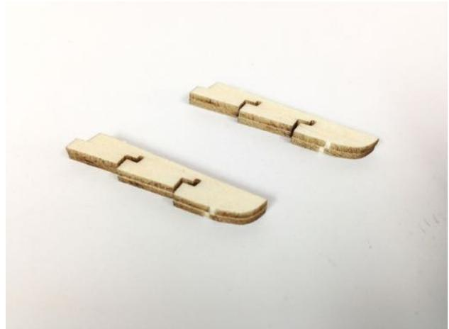
Exhausts - Laminate 2 exhaust parts EX to make each set of exhaust pipes.
