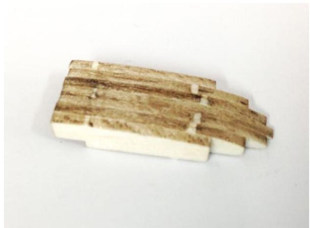
Air Inlet - Laminate parts A1, A2 and A3 in the order shown on the plan to make air inlet.
