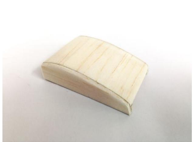
Radiator - Once set, sand to profile shown on the plan and bevel edges of RD1 to match the side profile.
