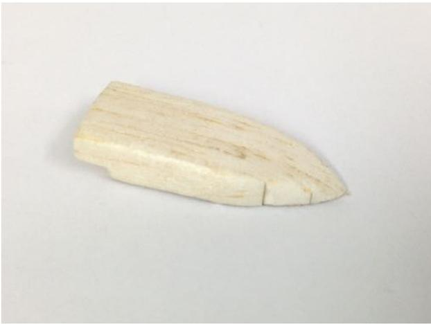
Air Inlet - Round of corners by sanding. You will need to sand the mating surface to match the belly fillet when fitting to the model later.
