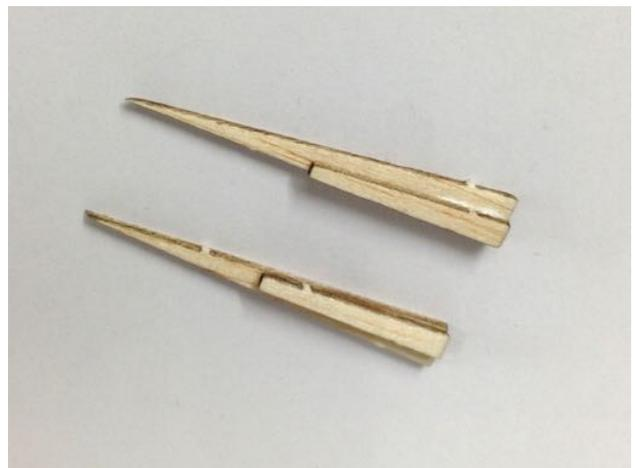
1) Continued: Make a left hand and a right hand fillet. These are sanded to fit on final assembly of the model.
