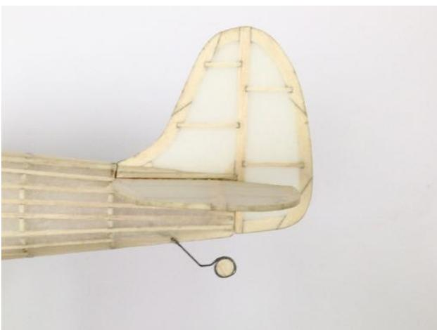
11) Noting the correct location of the tail wheel, make a pin hole in the tissue and glue in the tail wheel wire using epoxy.
