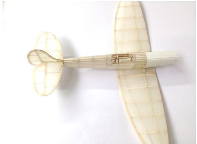
8) Glue the fin and rudder in place, ensuring it is properly located on the tail plane and at right angles to it.
