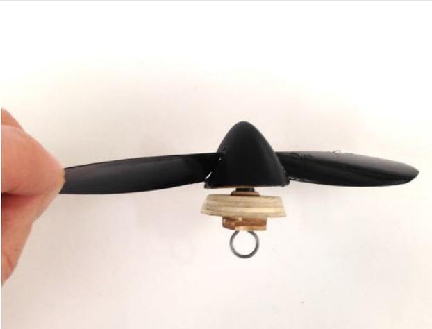
5) Continued: When you are satisfied, use quick setting epoxy to secure the spinner to the propeller blades with a neat glue fillet.
