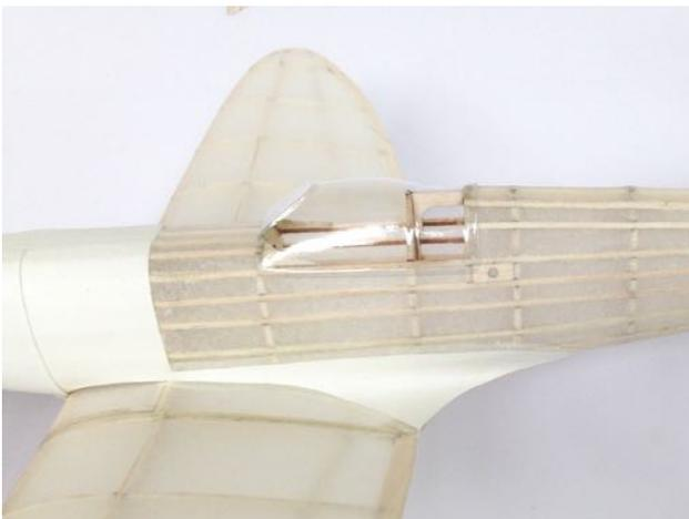
13) Fit one paper pattern U each side, curving them to fit along the wing, fuselage and WF, overlapping the tissue for a neat joint.
