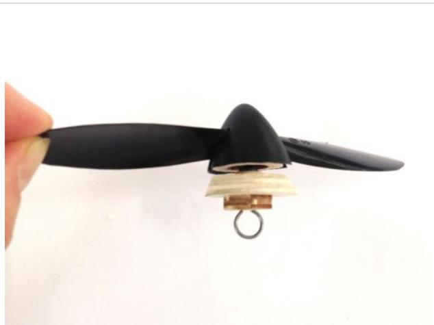
5) Continued: Now fit the spinner. The spinner should be trimmed so that it measures approx. 23mm from tip to rim. Cut two slots into the spinner to house the prop blades. The angled slots should finish approx 10mm from the spinner tip. Carefully tack the spinner in place with cyano, making sure that it does not wobble. **Do not get glue on the shaft or in the bush.**
