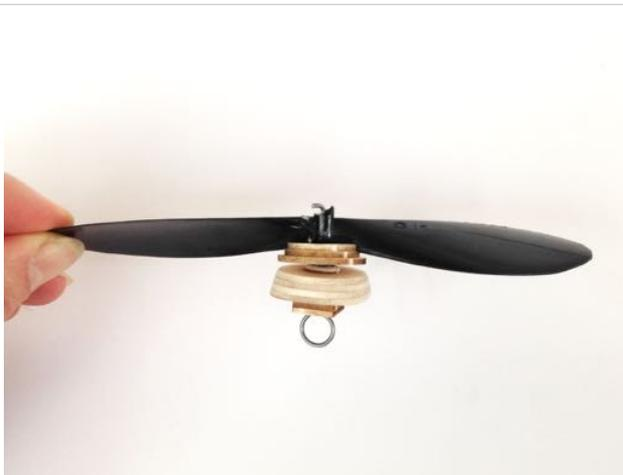
5) Assemble the propeller to the nose block using the wire prop hook as shown on the plan, making the shaft as short as possible.
