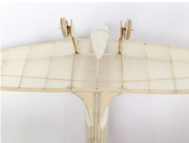
14) Cover the exposed side of parts WF, overlapping the tissue.
