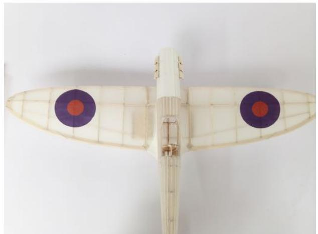
16) Markings are provided on lightweight paper; they should be cut out, and glued in position with a glue stick using the colour scheme diagram (Y) included at the back of the instruction booklet.
