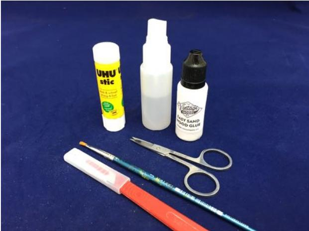
1) For the covering you will need a glue stick, PVA, fine brush, scissors, an old perfume bottle or fine mist sprayer and a sharp knife. It is also worthwhile to get a sponge and a dry cloth so that you can keep your fingers clean and dry as you work. Thin the PVA by around 50% with water (err on the strong side if unsure) in an old jar lid or similar.
