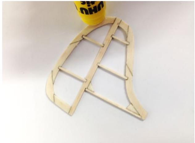
3) Continued: Lightly apply the glue stick only to the outside edges of the part. Keep the covering smooth and avoid it gathering in blobs on the surface and in corners.
