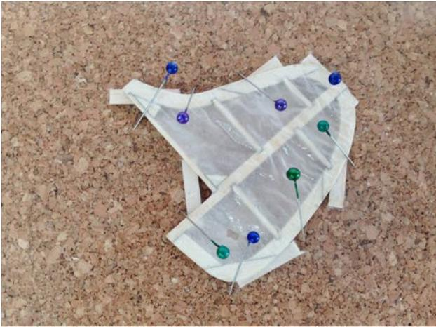
7) Spray the part with a fine mist of water on both sides, then use the spacers that you 'sticky taped' to hold the edge of the part off the board. Use pins set at an angle to hold it at until it dries. Holding the part down in this way helps prevent warps. Note the tissue is very delicate when it is wet, so handle the part at the edges and with care so that you don't damage it.
