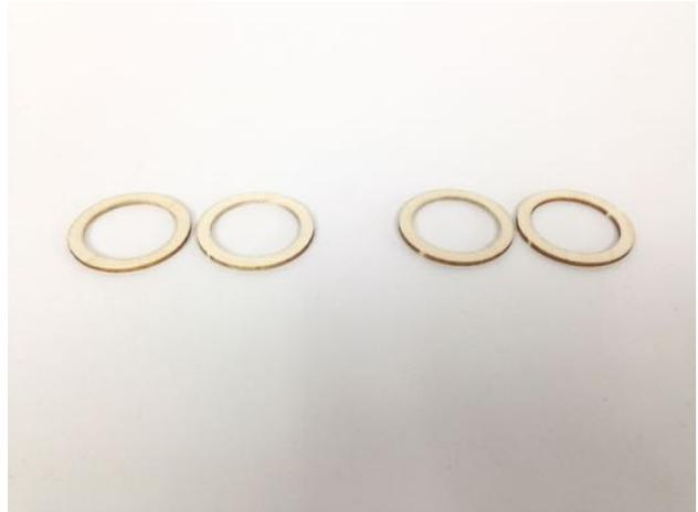
Sand the internal diameter of the WH1 and WH4 parts to remove the 'tags' and burnt edges using a piece of sandpaper wrapped round a pencil or similar.
