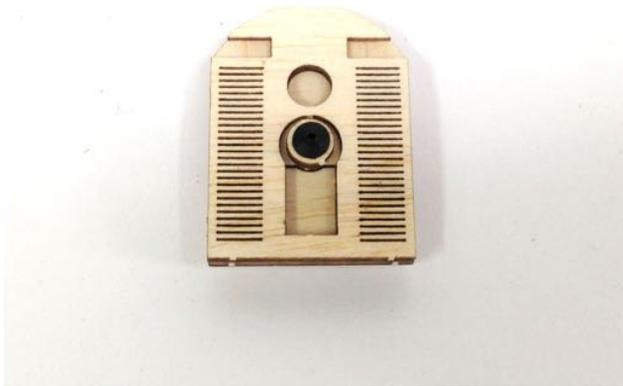
6) Glue a plastic nose bush into the hole in the nose block using cyano adhesive.
