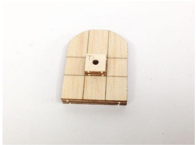
5) Glue the nose plug to the nose block, ensuring that it lines up with the cross markings on NB4 and that the holes remain in line. Make sure that any glue that squishes out between the parts is removed, otherwise it will prevent the parts from sitting together properly. Allow the completed nose block to dry.
