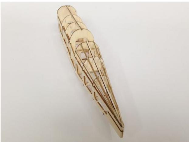
9) Fit and glue the remaining rear stringers, making them from light 1.6mm square strip, ensuring that the ends are bevelled to fit each other and the fuselage sides as instructed on the plan.
