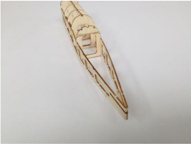
7)...Hold the ends together with a clothes peg or similar until the glue is set, then round off the end as shown on the plan.
