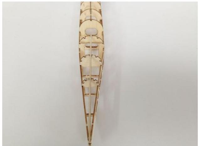
9) Using stiff 1.6mm square strip, fit and glue the 'backbone' stringer in position. Note that the end sits on top of the fuselage sides at the rear.
