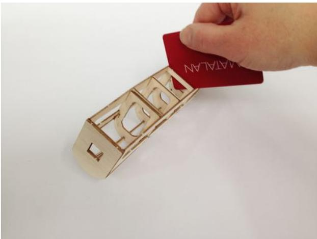
11) Continued... When gluing them in place, leave a gap of around 1mm (the thickness of a credit card) between them at the strengtheners on F3 and F5. This gap will accommodate the wire later.
