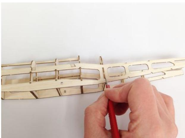
6) On the outside of each part K1, score about half the depth (not cut through) of the part along a line immediately behind F6, noted 'score line' on the plan. Each side should then be 'cracked' inwards forming a sharp kink in the side rather than a gentle bow.
