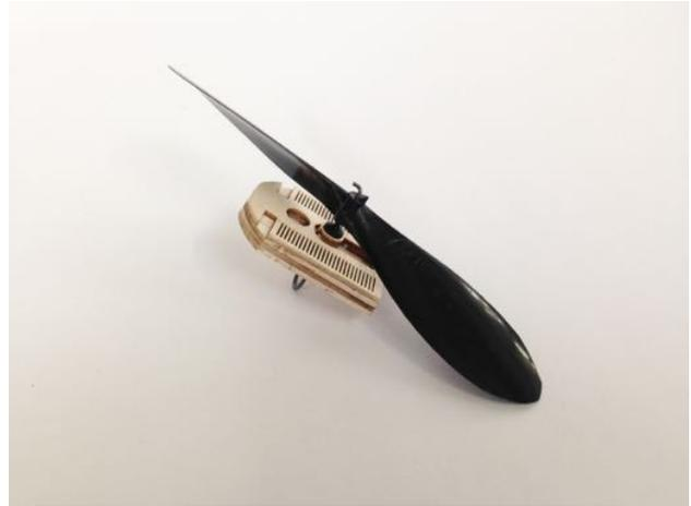
4) Assemble the propeller to the nose block using the wire hook as shown on the plan, making the shaft as short as possible.
