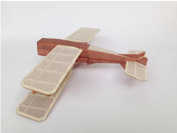
14) Glue the tail skid in place. N.B. this is a large part and forms a significant 'flying surface' so take equal care with this as with the fin etc. in making sure it is square and true.
