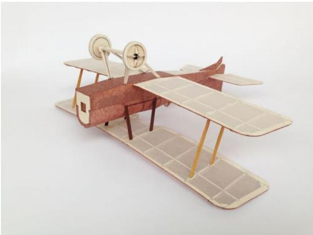
16) The wheels can then be added to the axles of the legs and retained by simply bending up the wire or using the insulations from some thin electrical flex held with a blob of glue. N.B. make sure that the glue does not enter the wheel centre bushing and the wheel can rotate freely.
