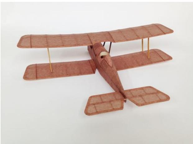
12) Glue the tail plane in position, making sure it is square, true and in line with the wings
