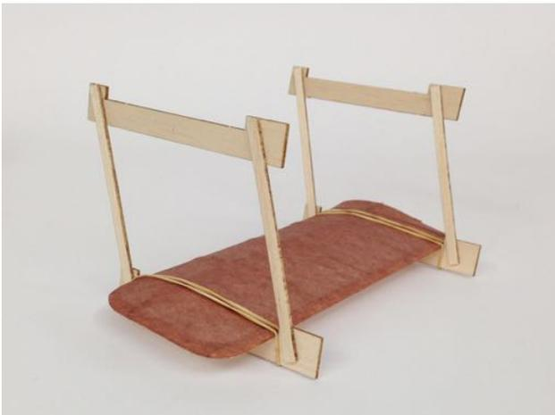
7) Once the glue on the cabane struts has dried, locate the left hand bottom wing to the top one using two wing decalage jigs. Use rubber bands to hold them in position.
