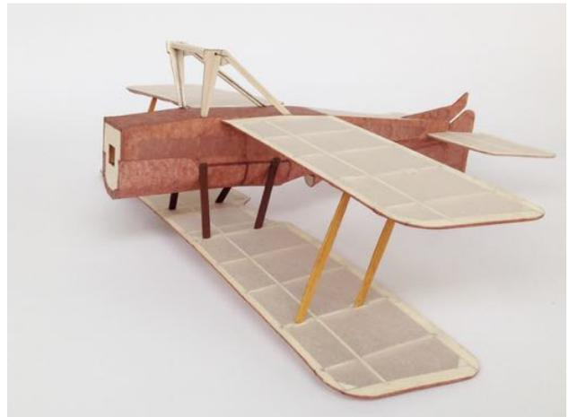
15) Make slits in the tissue at the positions of the F3 and F5 stiffeners – where the undercarriage wire will fit. Trial fit all of the undercarriage parts, bevelling the end of the LG4/LG4 assembly to fit snugly against the legs each side. Once a satisfactory fit is achieved glue all the parts together and to the fuselage using epoxy. Ensure good joints but do not use too much epoxy as it is quite heavy. Hold all the parts in position, square and true until the epoxy has set.
