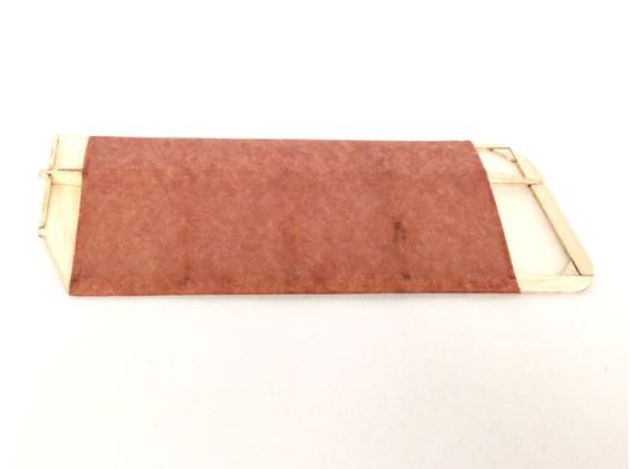
2) Cover the top in three pieces, the main wing panels from the root rib to the tip rib, then from the tip rib to the wing tip itself, and finally from R7 to the root rib.
