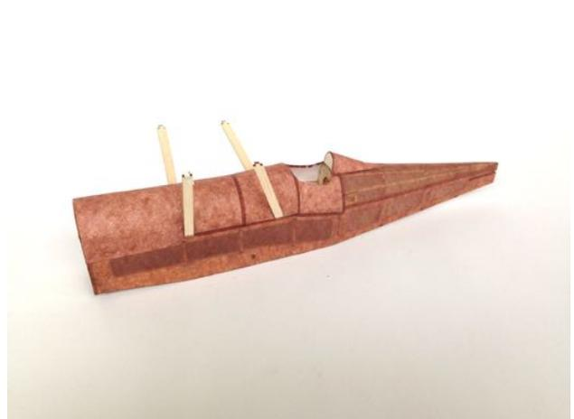
11) Continued Do not fold over any of the edges, instead use them to make neat overlaps when you fit the part from HR1 to the fuselage.
