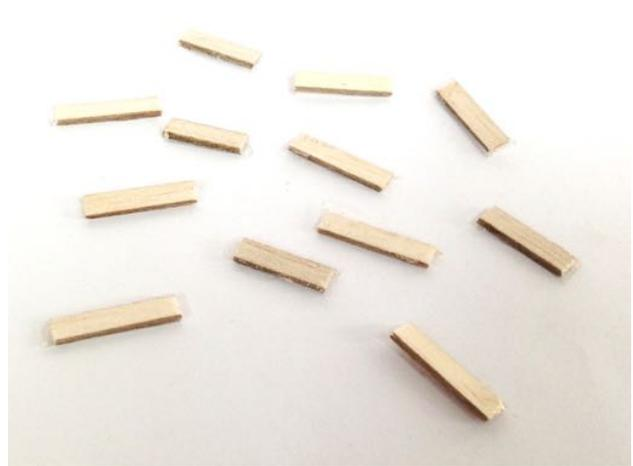
2) Cut out some spacers (about a dozen or so) about 20mm long and 5mm wide from the edges of the left over sheet and apply one layer of sticky tape to one surface. These spacers are used when shrinking the tissue – the sticky tape simply prevents the spacers sticking to the parts.
