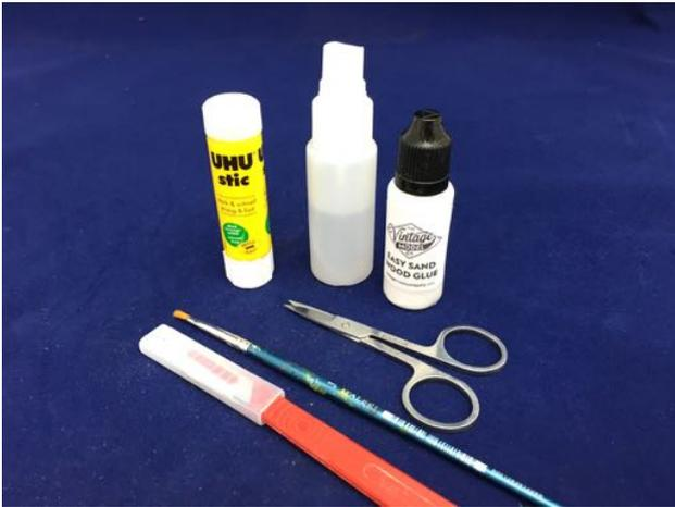
1) For the covering you will need a glue stick, PVA, fine brush, scissors, an old perfume bottle or fine mist sprayer and a sharp knife. It is also worthwhile to get a sponge and a dry cloth so that you can keep your fingers clean and dry as you work. Thin the PVA around 50% with water (err on the strong side if unsure) in an old jar lid or similar.
