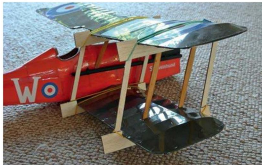
First the top wing is attached over a square reference and then the lower wings are glued in place using jigs.
