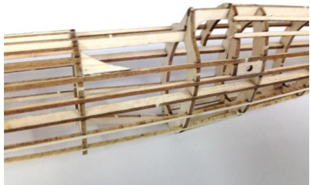
16) Continued: Then trial fit F17 bevelling the edges to meet the stringers each side to ensure a snug and flush fit to the outer profile. Glue it in position.
