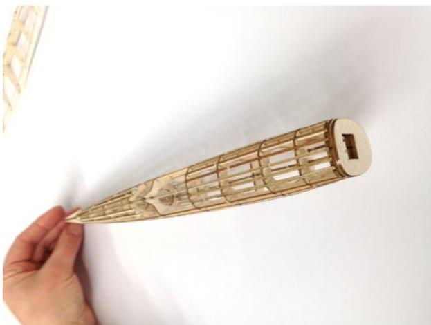
14) Now follow previous steps 5 -10 for this side, checking at each stage of adding a stringer that the fuselage is staying straight and true.
