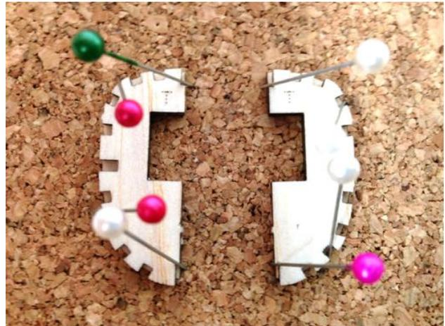
2) Make two opposite hand (ie one left hand, one right hand) laminations from parts F2 and F3, pinning them to the board to keep them flat and aligned. Ensure that the parts are orientated correctly by referring to the 'T' markings and that the rectangular cut out in each part lines up perfectly. Ensure any excess glue is removed from the slots in F3, otherwise the stringers added later may not fit. Leave the parts to dry thoroughly and remove from the board before proceeding.
