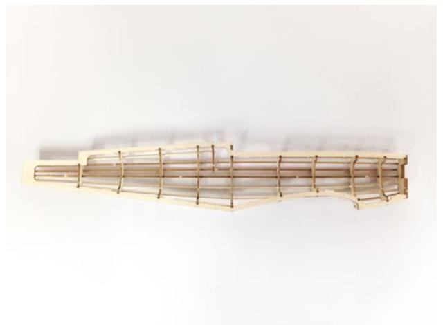
11) Allow everything to dry for as long as possible, then remove it from the board. Carefully cut out the five temporary crosspieces from the main keel.
