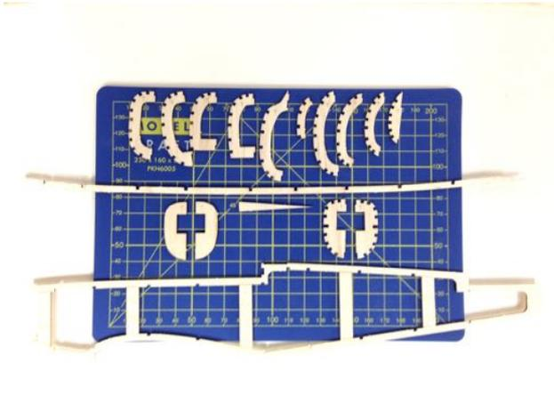
1) Identify and remove parts in the following quantities from the laser cut sheets: 1 off each: F4-F13, K2, and K4, plus: 2 off F2 and F3, and 1 off K1. Note that part K1 is quite delicate and large so carefully cut it from the sheets and handle it with care.
