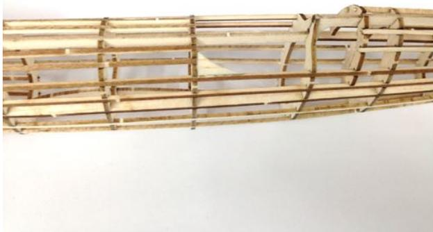
16) Starting with the left hand side, fit F14 tilting it to match the fuselage and former profile.
