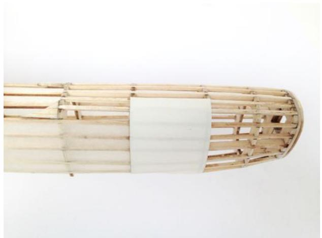
9) Fit the parts to the fuselage using a glue stick working from pattern Y forward overlapping them. They fit from F6 forwards and the stringer one down from the top keel, right round to the bottom keel. Use the tissue overlap at the bottom keel to make a good almost invisible joint.
