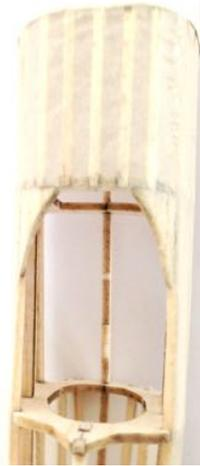
2 c) Cover top section in front of cockpit between F6 and F7 in one piece from Stringer "A" on one side to Stringer "A" on the other.
