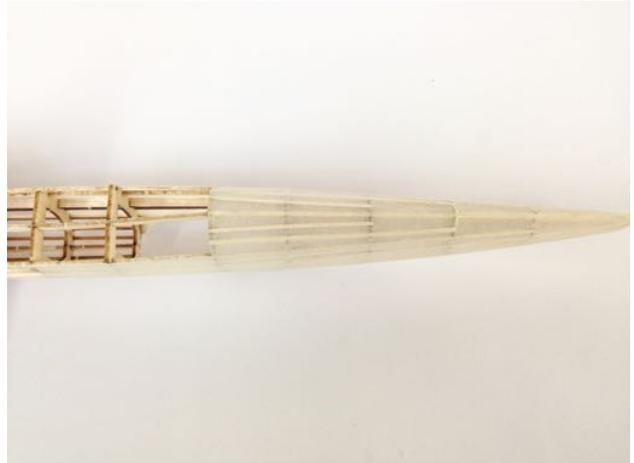
2b) The bottom area in one piece from side to side that runs from F8 to F12.
